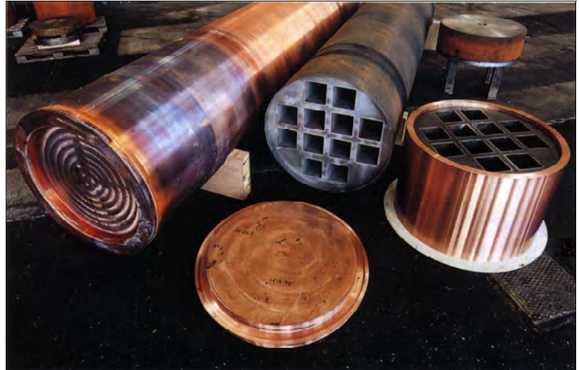
Figure 6.2. Example of fabricated canister components and objects (RD&D Programme 2001).
